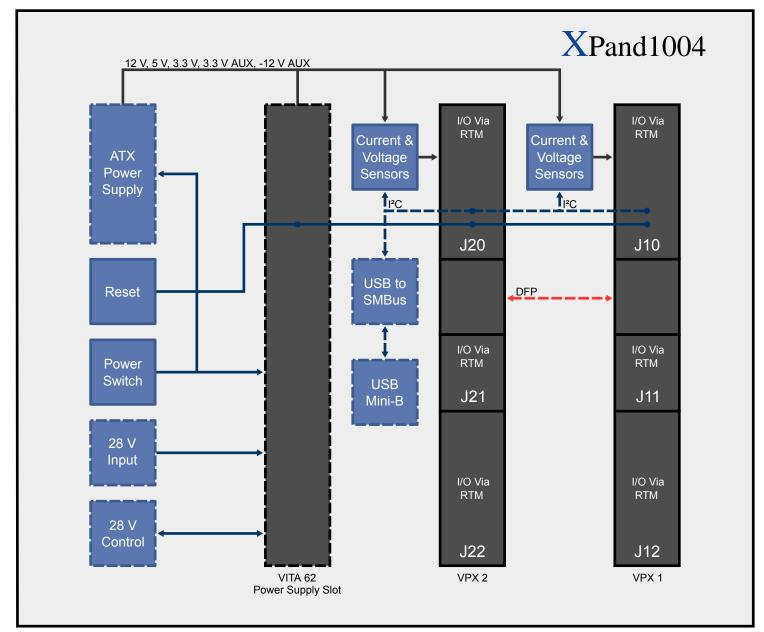
Dashed lines indicate configuration-specific functionality. Please contact X-ES Sales to determine the appropriate configuration to support desired functionality.
