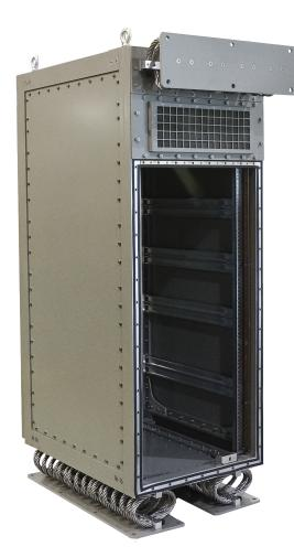
The MB-Series uses a modular base design which enables efficient cabinet reconfigurations. Common scalable components can be quickly adapted to a variety of cabinet sizes and feature sets. In certain applications, the bolt-together construction may enable multi-staged installation, where access is limited due to small passage ways and other obstructions.
